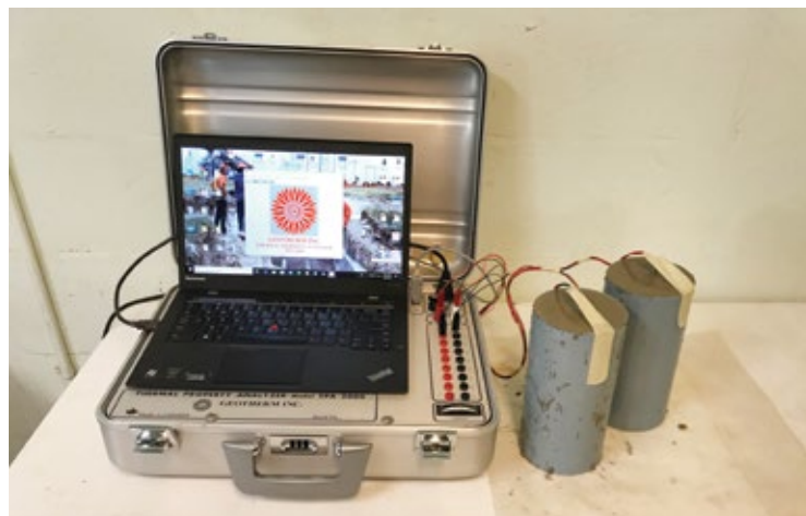
Figure 9. Thermal resistivity testing
