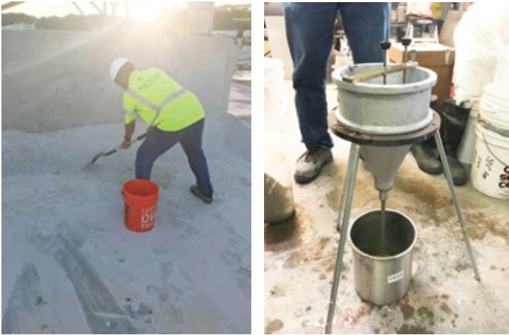
Figure 6. Material sampling and flow cone test
