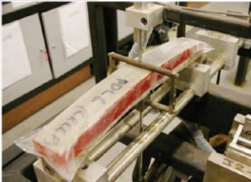
Figure 6: Wet Creep tests under load (Gumbel 2009)
