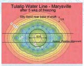
Figure 1: TEMP/W results for the inclined shaft after five weeks of freezing.
