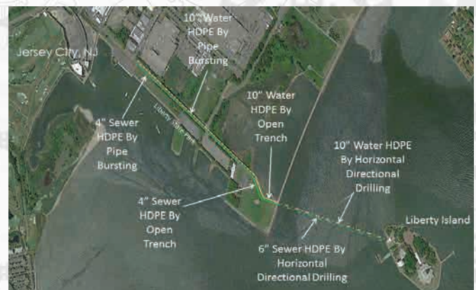
Figure 1: Location Plan and Installation Techniques
