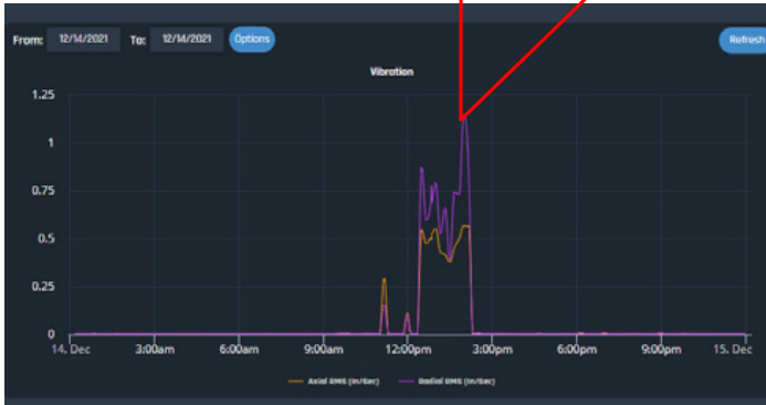
Figure 3 – PumpSentry Vibration Data log from the 100 MGD Bypass project where a significant manufacturing issue was determined. This graph shows the axial and radial vibration, with concern that the radial vibration is more than 1-inch per second
