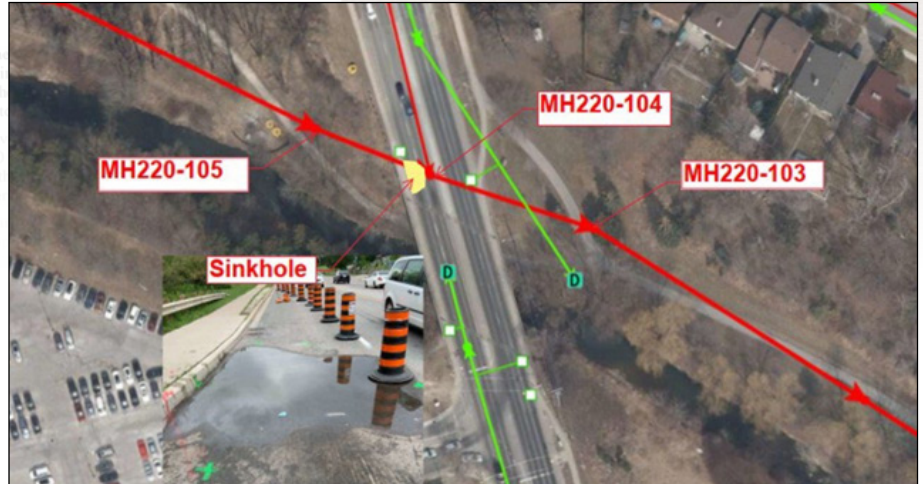
Figure 7. HCI Location Plan and Surficial Settlement/Sinkhole
