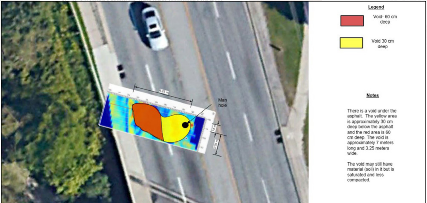
Figure 8. HCI GPR at Sinkhole Location
