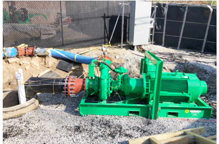
Figure 2 - 800hp - Electric Drive Pump
