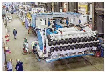
The MDM5000 (standing for Mine Development Machine with dimensions of  $5.0 \ m \ x \ 4.5 \ m$ ) is capable of excavating a flat tunnel invert in hard rock.
