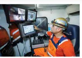
A crew member operates the MDM5000 in Fresnillo, Mexico from a state-of-the-art, air-conditioned control cabin using touch screen technology.
