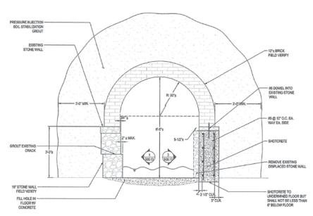
Figure 5. Example of specification drawings for Columbia Canal Tunnel Lining Project
