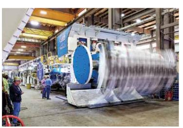
Developed by Robbins for use in rock up to 200 MPa UCS, the MDM5000 excavates with a reciprocating cutterhead and swinging cutterhead motion to create a rectangular cross section tunnel.
