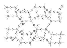
Figure 3. Example of aluminosilicate molecular geopolymer structure (Davidovits, 2011)
