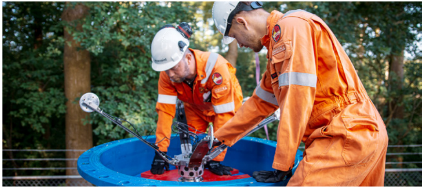
Acquaint's Acquirus in-line inspection tool with multi-sensor technology can be deployed in line with minimal to no system shutdown
