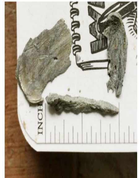
Figure 7. Photos of the pieces of metal found in the spoils coming off of the separation plant
