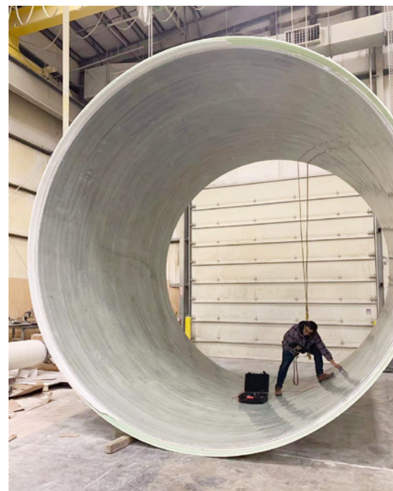
Figure 4. UT inspection on the 16-foot pipe with customized wave algorithms
