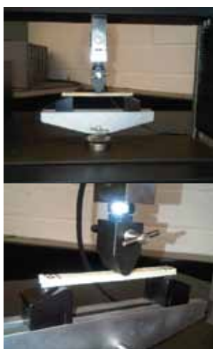
Bending testing in accordance with ASTM D790.
