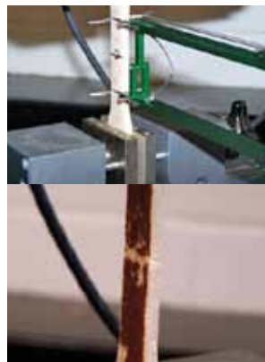
Tensile testing in accordance with ASTM D638. The specimen before the test (top) and after the test (bottom).
