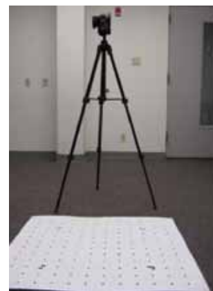
Figure 1: Camera setup for taking images for calibration
