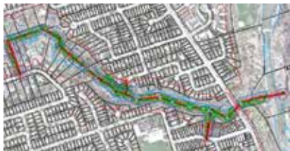
FIGURE 1 – Chapman Sanitary Trunk Sewer Alignment.
