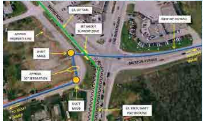
Figure 2 – Project alignment near manholes 6B and 7B. Traffic Management
