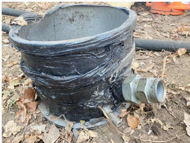
Steel manifold used in the steam curing process
