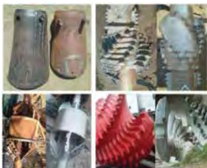
FIGURE 3 — Before and after photographs depicting abrasion of drill tools in dense glacial sand and gravel.
