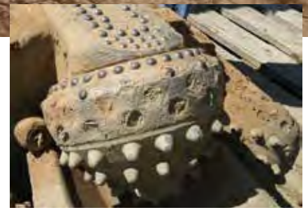
FIGURE 5 — Roller cone with shattered buttons. Note minimal abrasion in remaining button.
