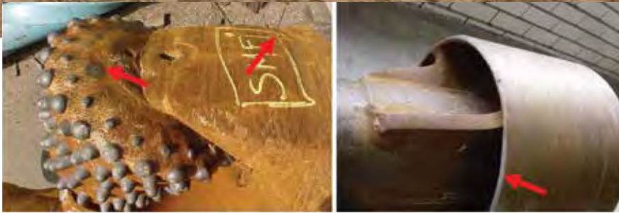
FIGURE 4 — Examples of tool abrasion resulting from tool gauging.
