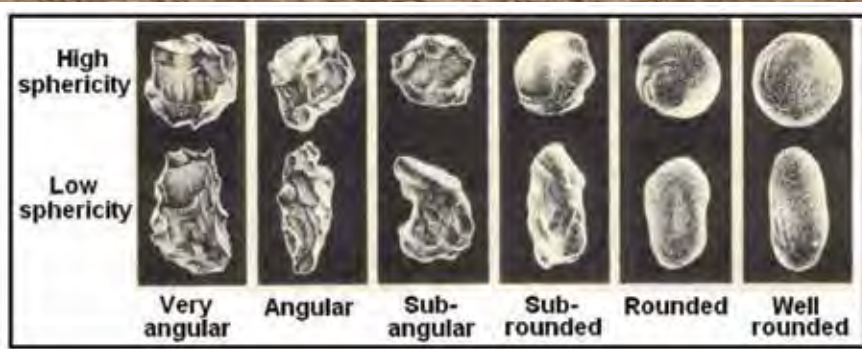
FIGURE 2—Sediment roundness scale of Powers, 1951.
